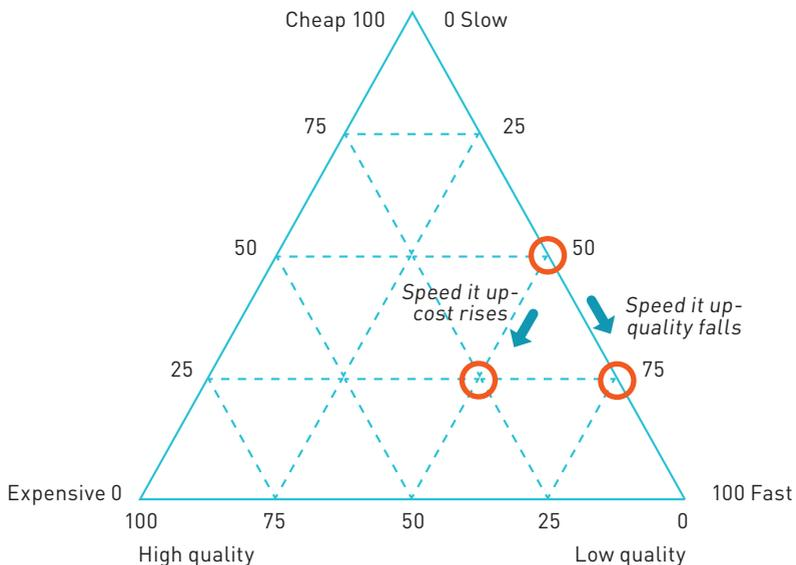
Figure 18 Two of the three characteristics cheap, fast, high quality are possible
